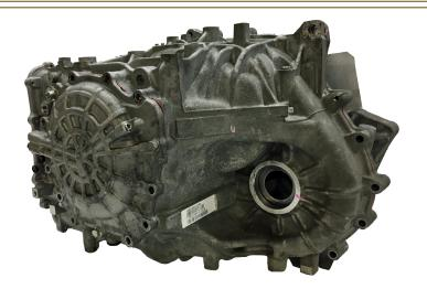
TransTec® overhaul kits #2726 and #2727 (with pistons) which service the 6F24 2012-UP 6 speed transmission are now available.
