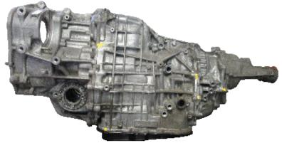
Now available TransTec® overhaul kit with pistons DP2697 which services the TR690 09-UP Subaru CVT transmission.
